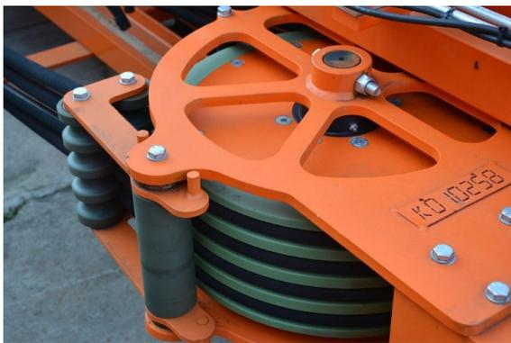
1. An external system can use much bigger pulleys than an internal system, as it has no limitation on space - big pulleys have a larger bending radius, with the resultant rope and hose life increase already mentioned above
